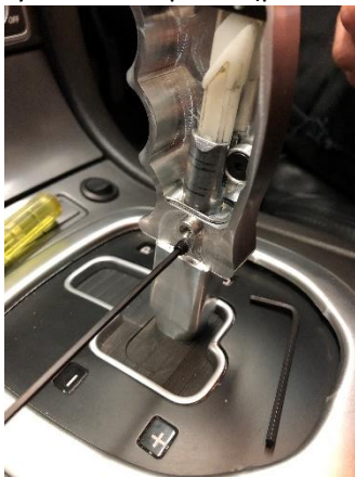
9. Tighten the grub screws on both sides as pictured. Before putting on side covers, ensure shifter works and shifts as required.
