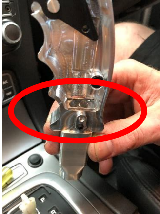
7. Install the original circlip removed in step 4, place clip in lower section of your new RipShift (please refer to photo)
