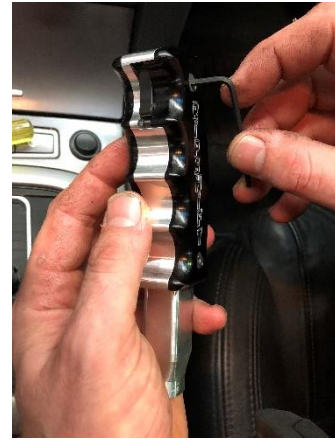
6. On your new RipShift, undo both side cover panels with supplied Allen key (2.5mm)
