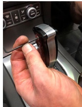
10. Place side covers and screw down with supplied Allen key
