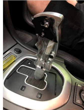
8. Slide shifter down (it may be firm) make sure clip goes over shaft and slide shifter down until it locks into place.
